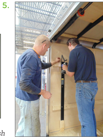
The bike trays are mounted on the 2x4" rails.
