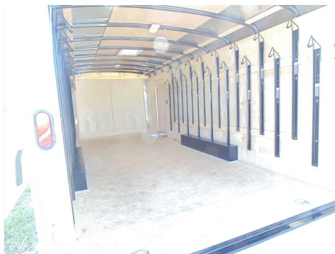
The interior finish may require notching to allow the rails to sit flush against the wall surface.
