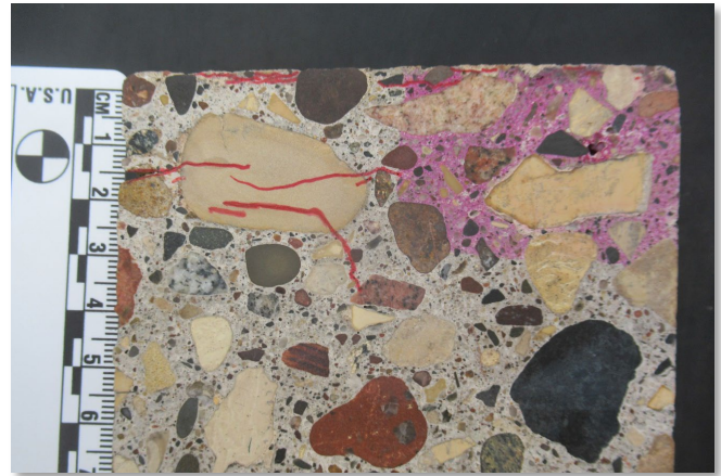
Exhibit 1. Concrete core petrographic analysis.
