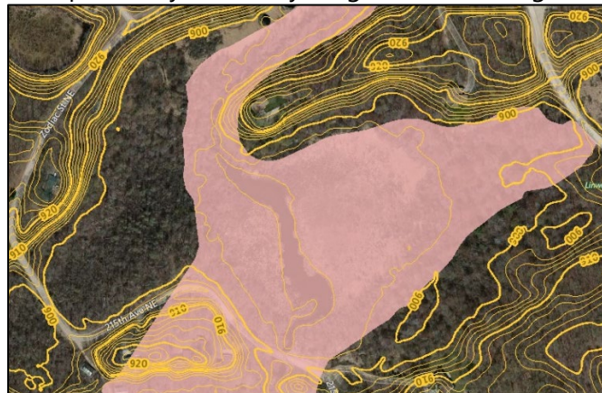
Figure 1: The mapped floodplain may not always align with on-the-ground contour elevations.
